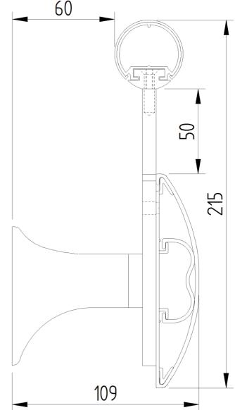
insert the cut 'closer' sections before fitting the handrail onto the wall. To minimise dirt traps all closer sections should leave a gap of no more than 2mm in the sections they are required to fill. Closer sections will not span a jointing block.
