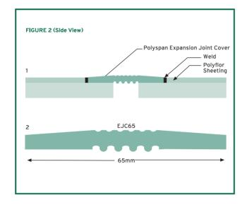
65 mm x 2 mm PVC Strip with a 20 mm expandable strip in the centre for application over filled expansion joint with a weld capability to the sheeting on either side of the expansion joint. Please see Figure 2.
