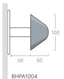
metal extender bracket up to 300mm (post cut to size)
