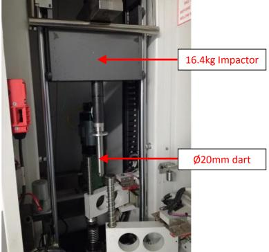
Rosand Impact Tester fitted with Ø20mm ball-nosed dart and an impactor mass of 16.4kg
