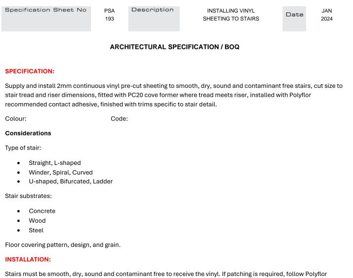
stairs must be smooth, dry, sound and contaminant free to receive the vinyl. If patching is required, follow Polyflor recommended patching compound supplier application instructions. Material must be installed in environmentally controlled conditions and must have been allowed to acclimatise for a minimum of 24-48 hours.
